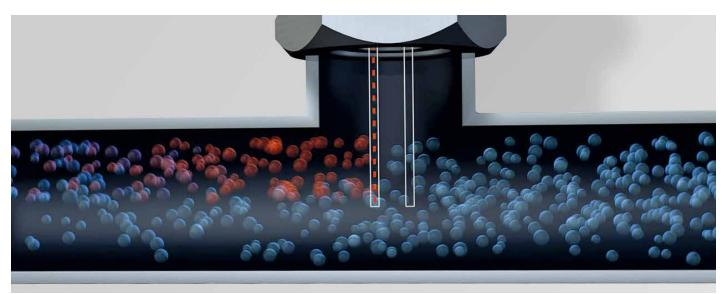
Two temperature sensors are installed in series in the direction of flow. The first temperature sensor measures the current process temperature of the compressed air, while the second sensor is electrically heated to a temperature that is 40 K higher than that of the first sensor.
